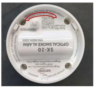
If you have a Sentech SK-20NZ Smoke Alarm installed which has started to sound the low battery warning, please check the back of your alarm for the recommended replacement date.
